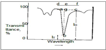
*Fig.4:* The BaselineMethod for Determining theAbsorbance of an Absorption *Maximum.*
