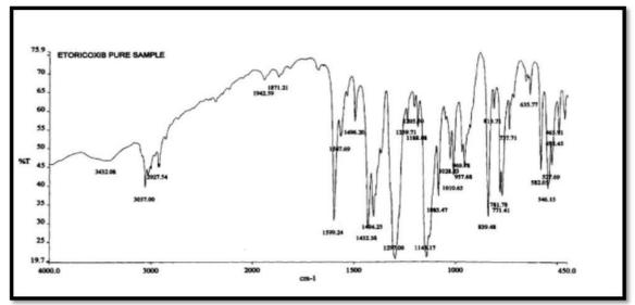
Fig.2: IR SpectrumofEtoricoxib.
