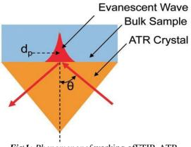
Fig1: Phenomenonof working of FTIR-ATR
